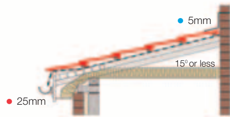
Cold roof abutment construction
